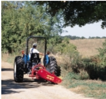
The mounted 451 has an exclusive telescoping yoke that uses tractor power to lift the mower.
